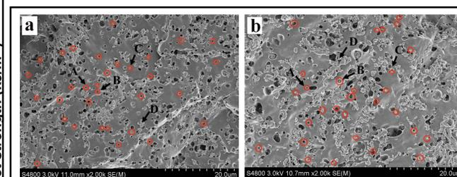
Fig. 7. SEM micrographs of different IPC samples. (a) *IPC-o*, (b) twice-extruded samples
