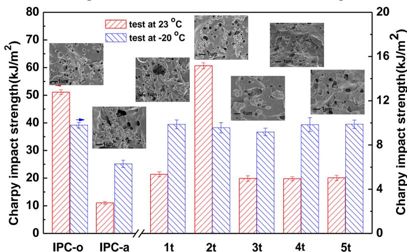
Fig. 6. Notched Charpy impact strength of *IPC-o*, *IPC-a* and samples after multiple extrusion.
