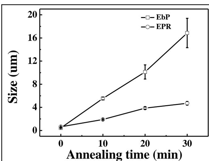
Fig. 3. Dispersed phase size of IPC samples annealed at 210 °C for different time.
