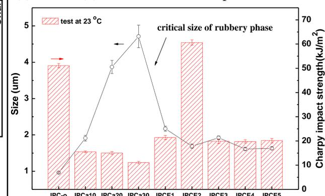
Fig. 8. Rubbery phase size and notched Charpy impact strength of different IPC samples
