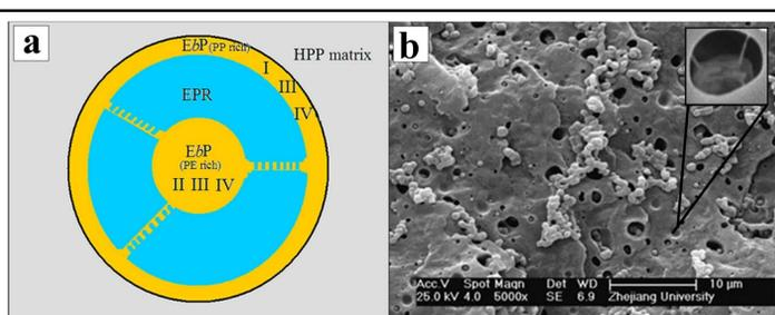
Fig. 1. Phase structure model of IPC and SEM micrograph of dispersed phase.
