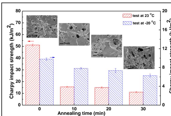
Fig. 4. Notched Charpy impact strength of IPC samples annealed at 210 °C for different time.
