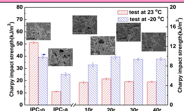
Fig. 5. Notched Charpy impact strength of *IPC-o*, *IPC-a* and samples after extrusion with different rotate speed.
