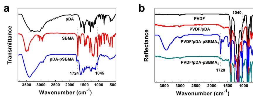
Figure 2. FTIR spectra of (a) synthesized pDA-pSBMA and (b) PVDF/pDA-pSBMA membranes.
