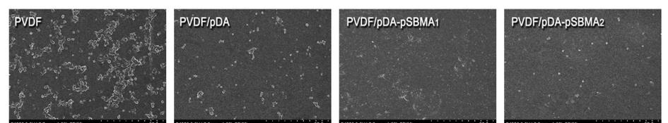
Figure 5. Morphologies of platelets on pure and modified PVDF membranes.
