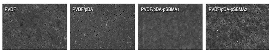
Figure 3. Surface SEM images of pure PVDF, PVDF/pDA and PVDF/pDA-pSBMA membranes.
