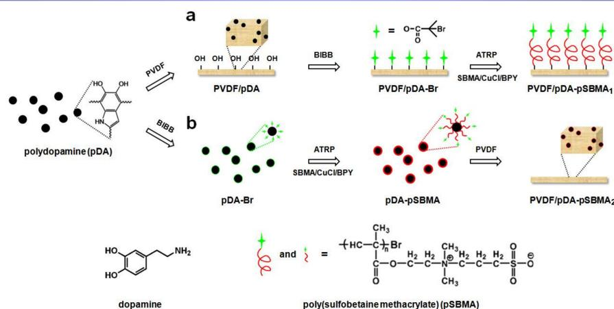
Figure 1. Scheme for preparation of PVDF/pDA-pSBMA membranes via two methods.
