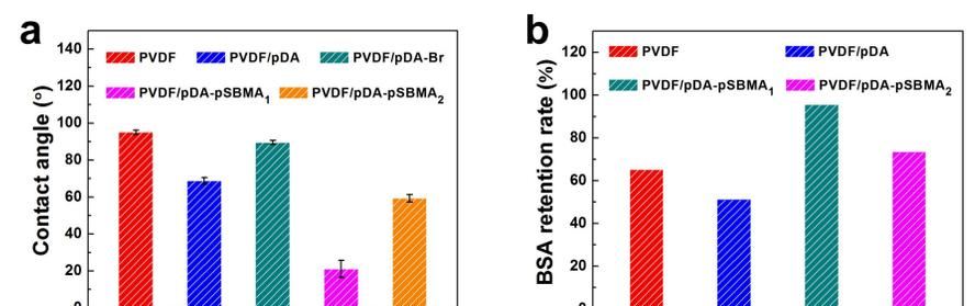
Figure 4. (a) Contact angle and (b) BSA retention of pure and modified PVDF membranes.
