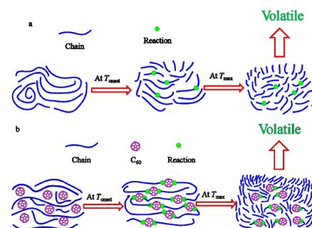
Fig. 3 Schematic representation of the mechanism for the thermal degradation of HDPE/ $C_{60}$  nanocomposites in  $N_2$ : (a) the thermal degradation process of HDPE; (b) the thermal degradation process of HDPE/ $C_{60}$  nanocomposites.
