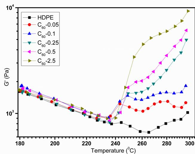
Fig. 2 Dependence of storage moduli ( $G'$ ) on temperature for HDPE and HDPE/ $C_{60}$  nanocomposites.
