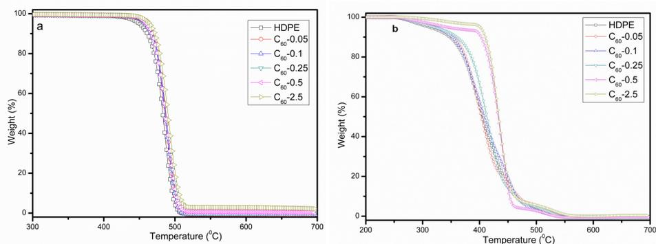
Fig. 1 TG curves for pure HDPE and HDPE/ $C_{60}$  nanocomposites in  $N_2$  (a) and air (b)
