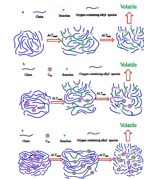
Fig. 4 Schematic representation of the mechanism for the thermal degradation of HDPE/ $C_{60}$  nanocomposites in air: (a) the thermo-oxidative degradation process of HDPE; (b) the thermo-oxidative degradation process of HDPE with low concentration of  $C_{60}$ ; (c) the thermo-oxidative degradation process of HDPE with high concentration of  $C_{60}$ .
