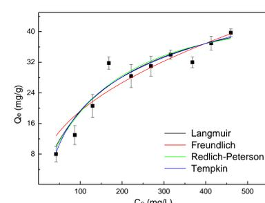
**Figure 6.** Adsorption isotherm fitted with Langmuir (black line), Freundlich (red line), Redlich-Peterson (green line), and Tempkin (blue line) models for the adsorption of mesoporous PTMSPMA in BSA acetate buffer solutions at room temperature.
