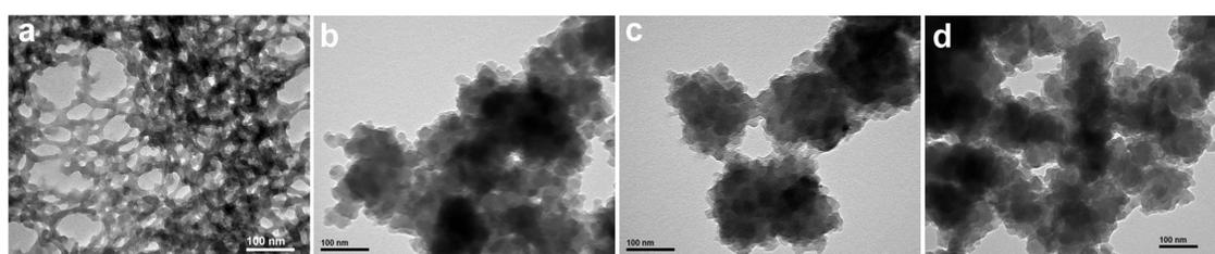
**Figure 1.** TEM images of the resultant mesoporous polymers. (a) PTMSPMA, (b) PTS-15, (c) PTS-5, and (d) PTS-2.
