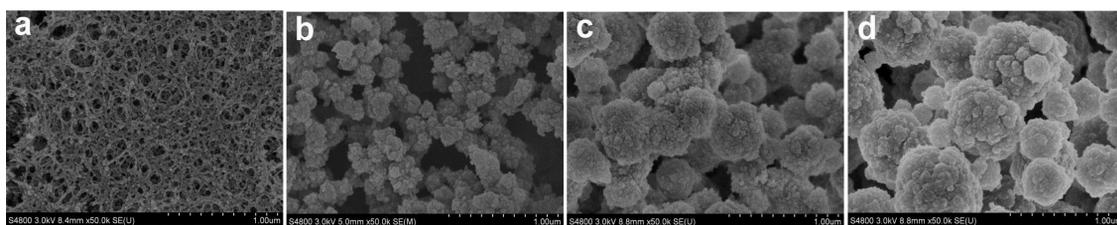
**Figure 2.** SEM images of the resultant mesoporous polymers. (a) PTMSPMA, (b) PTS-15, (c) PTS-5, and (d) PTS-2.
