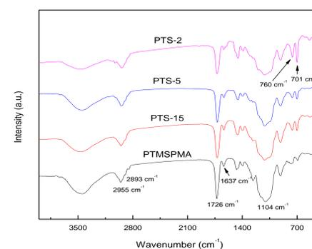
**Figure 3.** FT-IR spectra of the resultant hybrid mesoporous polymers, i.e. PTMSPMA, PTS-15, PTS-5, and PTS-2.
