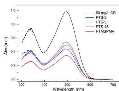
**Figure 5.** The UV spectra of filtered mixed solutions after mixing PTS-2, PTS-5, PTS-15, and PTMSPMA, respectively, in the 50 mg/L congo red (CR) aqueous solutions for 24 hrs.
