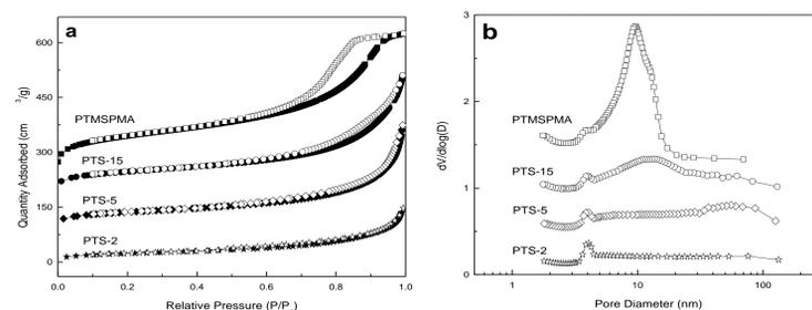
**Figure 4.** (a) Nitrogen adsorption-desorption isotherms of PTMSPMA, PTS-15, PTS-5, and PTS-2. (b) Barret-Joyner-Halenda (BJH) pore size distributions calculated from the corresponding desorption data in (a).
