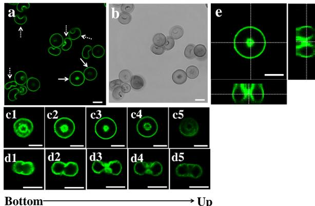
**Fig. 2** CLSM image (a) and transmission mode image (b) of RBC-like microcapsules with a diameter of  $\sim 6.7 \mu\text{m}$  in water. Series Z-scanning CLSM images of the typical RBC-like microcapsules (c) lying and (d) standing on the substrate, respectively. (e) 3D reconstruction of the microcapsule shown in (c). Scale bar:  $5 \mu\text{m}$
