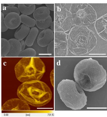
**Fig. 1** (a) SEM image of RBC-like  $\text{Ca}(\text{OH})_2$  particles with a diameter of  $\sim 6.7 \mu\text{m}$  and thickness of  $\sim 2.8 \mu\text{m}$ . (b) SEM and (c) AFM images of collapsed  $(\text{PAH}/\text{GA})_{10}$  microcapsules after being dried in air. (d) SEM image of  $(\text{PAH}/\text{GA})_{10}$  microcapsules dried by critical point drying method. Scale bar:  $5 \mu\text{m}$ .
