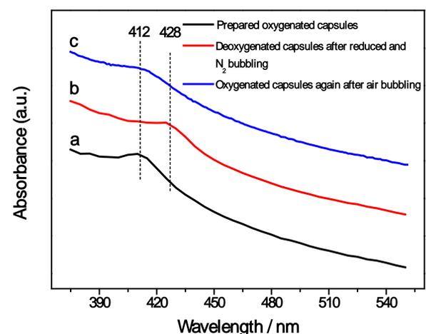
**Fig. 4** UV-vis absorption spectra of RBC-like capsules coated with Hb. (a) The prepared capsules in oxygenated states, (b) capsules in deoxygenated state after reduced by sodium dithionite and  $\text{N}_2$  bubbling, and (c) capsules in oxygenated state after air bubbling following  $\text{N}_2$  bubbling.
