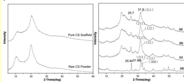
Fig.5 XRD patterns of raw material, pure CS scaffold, and CS/HA composite scaffolds: (a) CS/HA5; (b) CS/HA10; (c) CS/HA15; (d) HA (homemade)
