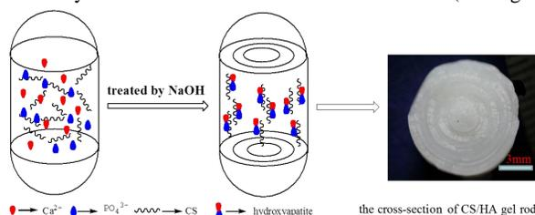
Fig.1. Scheme of the formation mechanism of CS/HA scaffolds
