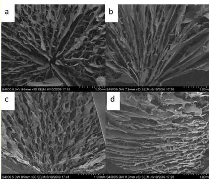
Fig.2 The SEM micrographs of cross-section (a, b, c) and vertical-section (d) of the scaffolds : (a)CS/HA5; (b) CS/HA10; (c) CS/HA15; (d) CS/HA10
