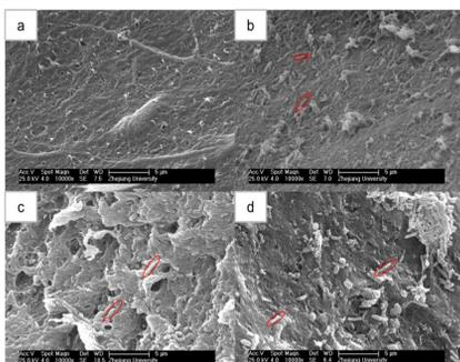
The CS/HA scaffolds exhibited a uniform interconnected open pore microstructure and a spoke-like, multilayer and porous structure from Fig.2. The Nano-HA were seen on the scaffold pore walls and were homogeneously dispersed in the matrix form Fig.3. The size of the crystal HA is about 50-500 nm with acicular shape and increased with the content of HA precursor.
