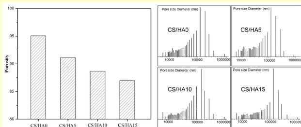
Fig.4 Porosity and Pore size Diameter of CS/HA scaffolds
