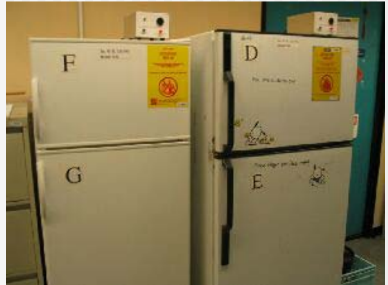
Explosion-proof Refrigerator: Storage of hazardous chemical
