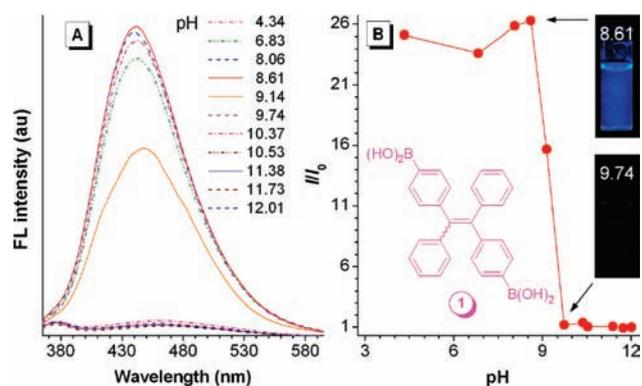
**Figure 1.** (A) FL spectra of **1** ( $10\ \mu\text{M}$ ) in Britton–Robinson buffers containing 2 vol % DMSO at different pH values. (B) Change in the FL intensity ( $I$ ) of **1** at 440 nm with pH;  $I_0$  is the intensity at pH 12.01. Inset: photographs of the mixtures of **1** in the aqueous buffers at pH 8.6 and 9.7 taken under the illumination of a hand-held UV lamp ( $\lambda_{\text{ex}} = 365\ \text{nm}$ ).
