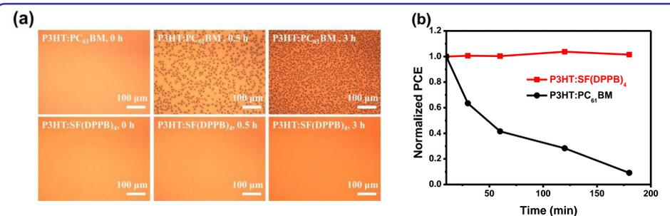
**Fig. 4** (a) Optical microscopy images showing morphological stability of P3HT:PC<sub>61</sub>BM (1:0.8, by wt.) and P3HT:SF(DPPB)<sub>4</sub> (2:1, by wt.) blended films after thermal treatment at 150 °C for various time; (b) graph showing the stability of the PCEs for the devices based on P3HT:SF(DPPB)<sub>4</sub> (2:1, by wt.) and P3HT:PC<sub>61</sub>BM (1:0.8, by wt.) blended films after thermal treatment at 150 °C for various time.
