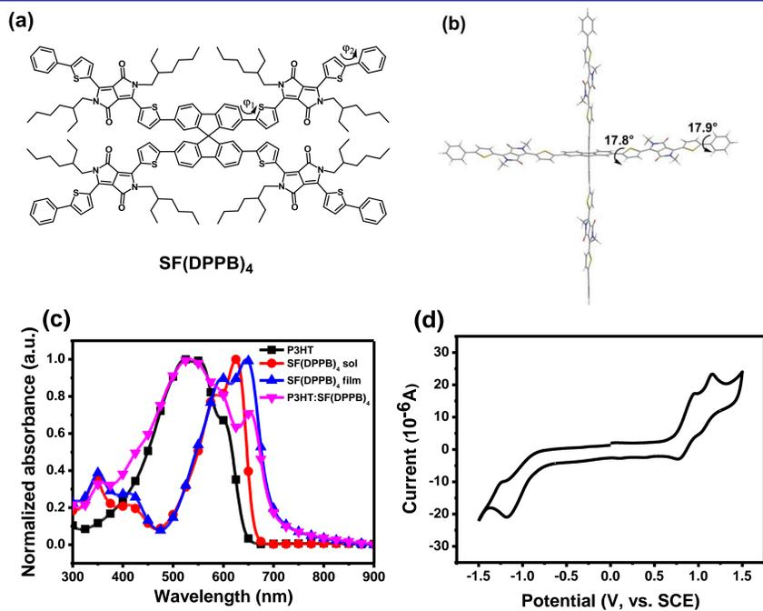
**Fig. 1** (a) Chemical structure of SF(DPPB)<sub>4</sub>; (b) ground-state geometry of SF(DPPB)<sub>4</sub> calculated by DFT method; (c) UV-vis absorption spectra of P3HT film, SF(DPPB)<sub>4</sub> solution and film, and P3HT:SF(DPPB)<sub>4</sub> (2:1, by wt.) blended film; (d) cyclic voltammogram for SF(DPPB)<sub>4</sub> in dichloromethane solution.
