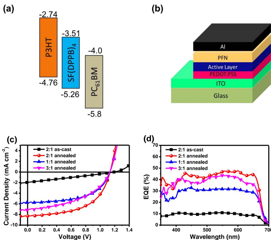
**Fig. 2** (a) Energy levels of P3HT, SF(DPPB)<sub>4</sub> and PC<sub>61</sub>BM; (b) the diagram of device structure; (c) J-V curves of PSCs with the structure of ITO/PEDOT:PSS/P3HT:SF(DPPB)<sub>4</sub>/PFN/Al; (d) EQE spectra of P3HT:SF(DPPB)<sub>4</sub> based PSCs.
