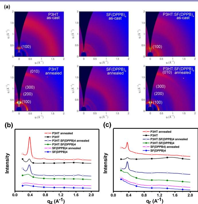
**Fig. 3** (a) 2D GIWAXS images of P3HT, SF(DPPB)<sub>4</sub> and 2:1 P3HT:SF(DPPB)<sub>4</sub> thin films with or without the thermal annealing at 120 °C for 10 min; (b) intensity profiles along q<sub>z</sub> axis of P3HT, SF(DPPB)<sub>4</sub> and 2:1 P3HT:SF(DPPB)<sub>4</sub> thin films; (c) corresponding intensity profiles along q<sub>r</sub> axis.
