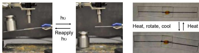
Fig. 6. Pictures showing the reversible bonding/debonding behavior and the shape-memory adhesive healing characteristics of the systems. 2
