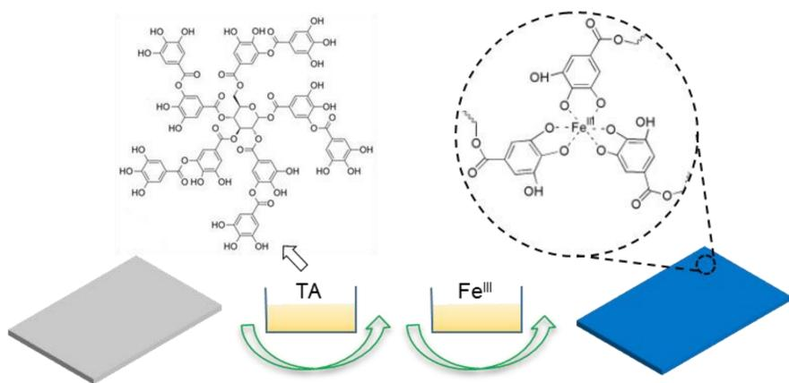
Figure 1. Schematic description of the preparation of the TA/Fe modified PP separator.
