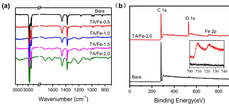
Figure 2. Spectra of (a) ATR-IR and (b) XPS for the bare and TA/Fe coated separators.
