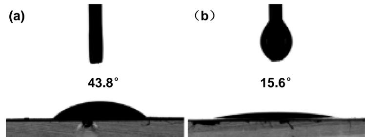
Figure 4. Liquid electrolyte contact angles for (a) the bare and (b) TA/Fe-2.0 separators.
