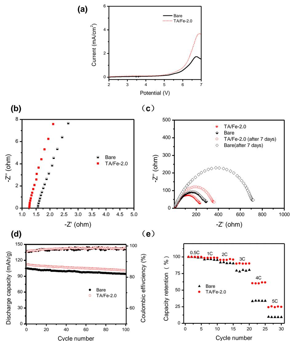
Figure 5. (a) I-V curves of the different separators in SS/separator/Li cells, impedance spectra of the (b) SS/separator/SS cells and (c) Li/separator/Li cells with different separators, (d) the discharge capacities and coulombic efficiencies of the cells as function of cycle number at 0.5 C and (e) rate capacities of the cells.
