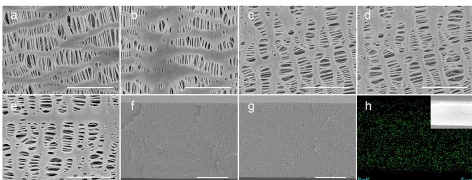
Figure 3. SEM images for (a-e) the surfaces of the bare and TA/Fe modified separators with the TA concentrations of 0.5 mg/ml, 1.0 mg/ml, 1.5 mg/ml and 2.0 mg/ml, respectively, and (f-g) cross section of the bare and TA/Fe-2.0 separators. (h) EDX mapping of the Fe element on the cross section of TA/Fe-2.0 separator.
