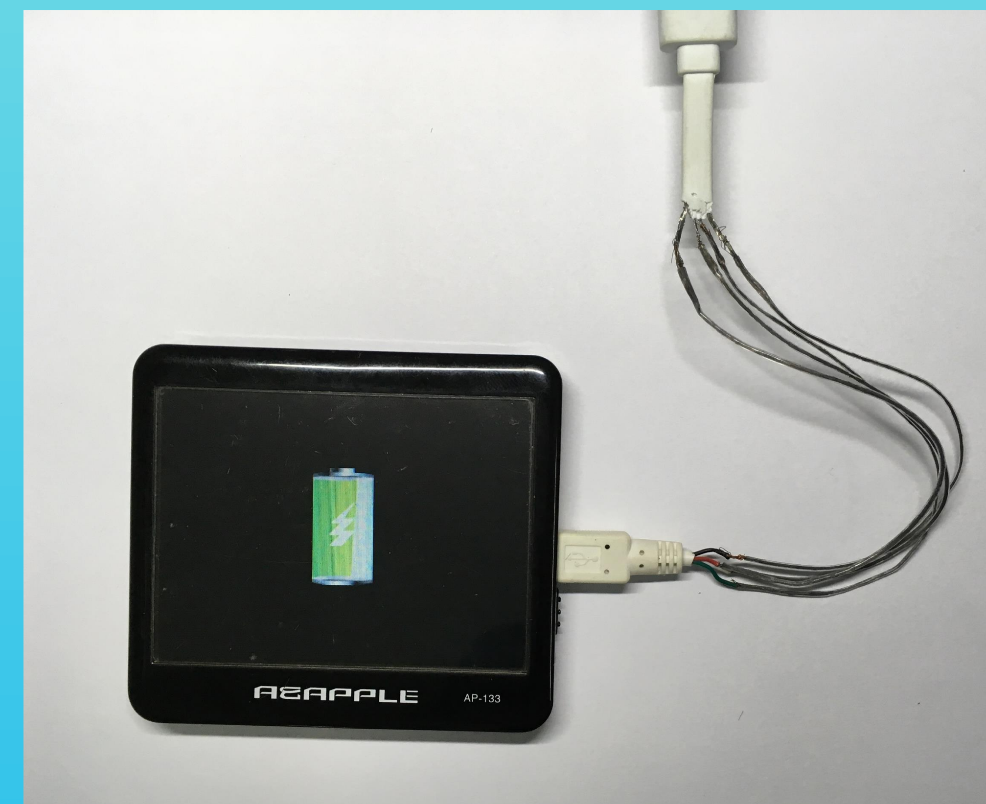
Figure 4. Applications of GFs to replace copper as long conducting wires, lightweight rotator coils, and USB cables.
