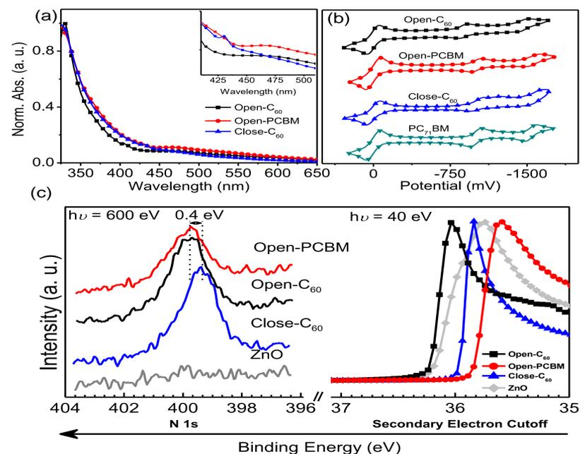
Figure 2. UV-vis absorption and CV curves of different fullerene, and Photoemission spectroscopy of ITO/ZnO with and without modification.
