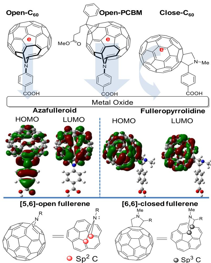
Figure 1. Schematic illustration of electron transport from fullerene interfacial modifier to ZnO (top), the modeled HOMO/LUMO (middle), and the structure difference of [5,6]-open fullerene and [6,6]-closed fullerene.
