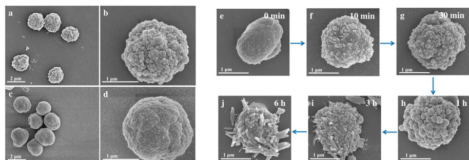
**Figure 1.** (a-d) SEM images of MP-NPs and MPs, which are prepared by incubating PAH-g-Por microparticles in pH 1 HCl for 1 h (a, b) and 0 min (c, d), respectively. (e-j) SEM images showing the process of nanoparticles protruding on the surface of PAH-g-Por microparticles and turning into nanorods, which are incubated in pH 1 HCl for 0 min (e), 10 min (f), 30 min (g), 1 h (h), 3 h (i) and 6 h (j), respectively.
