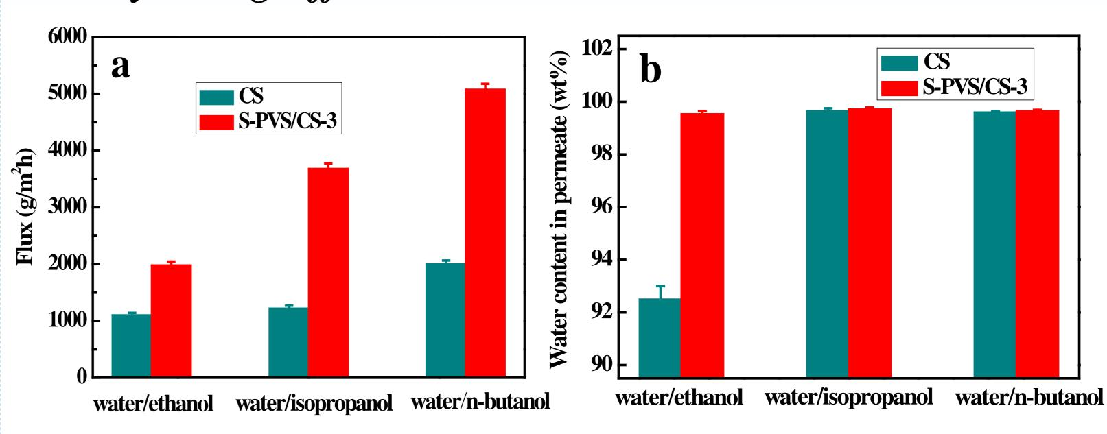
Permeate flux (a) and water content in permeate (b) of CS and S-PVS/CS-3 PECM in dehydrating 10 wt% water/ethanol, water/isopropanol and water/n-butanol mixtures, respectively, at 70oC.
