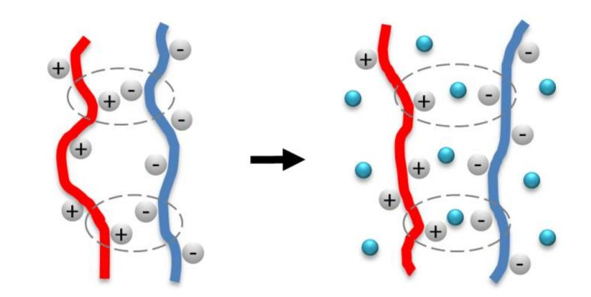
**Figure 4.** Simplified mechanism of how the water uptake affects the interactions between PEI and PAA. The effect of water can significantly disrupt the cross-linked network and activate the motion of the whole polymer chains. The red line and the blue line respectively represent PEI and PAA; the blue dots correspond to the water molecules within the film.
