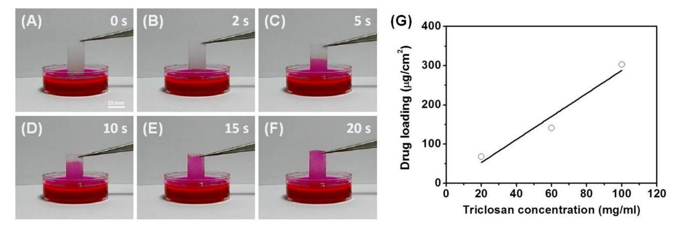
**Figure 2.** (A-F) Nile red, a hydrophobic dye, could be loaded into the microporous PEM film by wicking from its ethanol solution, indicating the presence of abundant open pores across the whole film. (G) Plot of actual triclosan loading with respect to the concentration of triclosan-ethanol solution.
