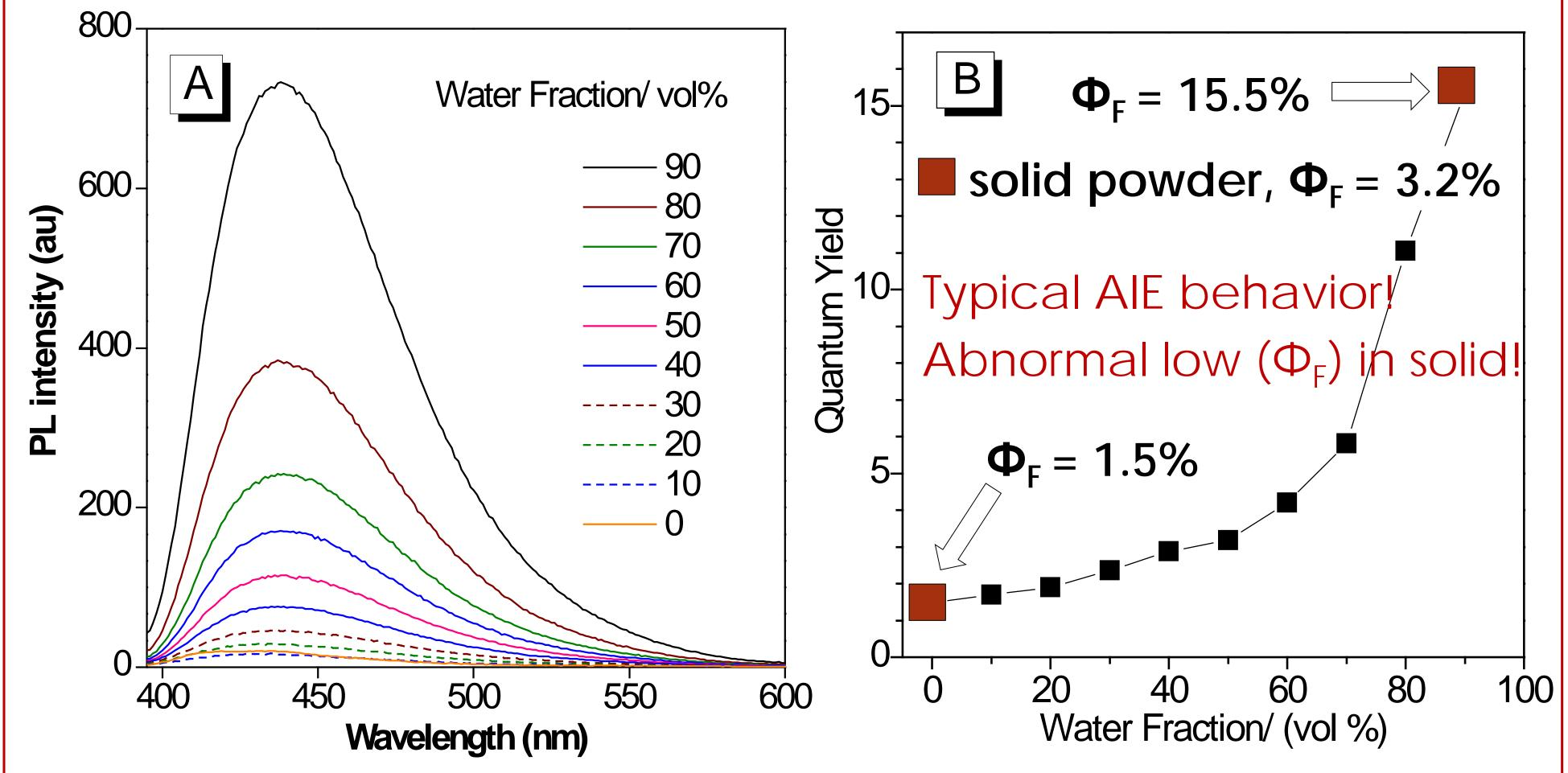
Fig. 3. (A) Photoluminescence (PL,  $\lambda_{\rm ex}$  = 375 nm) spectra of Box in DMSO/H<sub>2</sub>O mixtures with different H<sub>2</sub>O fractions ( $f_{\rm W}$ ). (B) Changes in PL quantum yield ( $\Phi_{\rm F}$ ) in DMSO/H<sub>2</sub>O mixtures. [Box] = 10  $\mu$ M.
