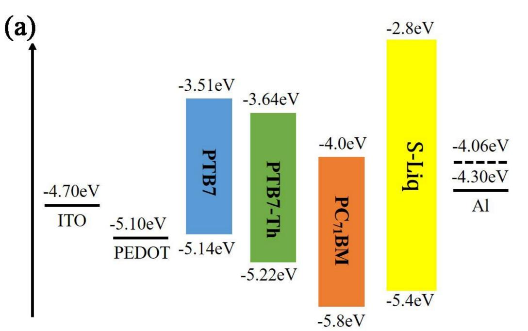
➤ Introducing s-Liq interlayer can provide strong electric dipole between the Al electrode and active layer
