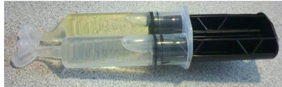
A syringe of "5-minute" epoxy, containing separate compartments for each of the two components
