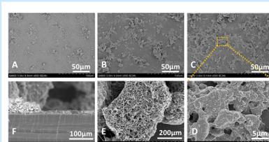
**Figure 6.** SEM images of the surface morphology and cross section of [PEI/(CNTs@PDA+ $\text{Fe}^{3+}$ )] multilayer films with 20 BL (A), 30 BL (B) and 50 BL (C, D, E, F, with different magnification).
