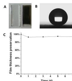
**Figure 7.** (A) Photographs of glass slide substrates uncovered (left) and covered with the sprayed [PEI/(CNTs@PDA+ $\text{Fe}^{3+}$ )] multilayer film (right). (B) Contact angle ( $150.9^\circ \pm 0.3^\circ$ ) of the film surface. (C) Thickness of the [PEI/(CNTs@PDA+ $\text{Fe}^{3+}$ )] multilayer film incubated in 150 mM EDTA for a week.
