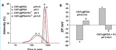
**Figure 3.** Size (A) and Zeta potential (B) of the particles in solutions of CNTs@PDA without  $\text{Fe}^{3+}$  at pH 8.5 (a) and 3 (b), and with  $\text{Fe}^{3+}$  at pH 3 (c) and 8.5 (d).
