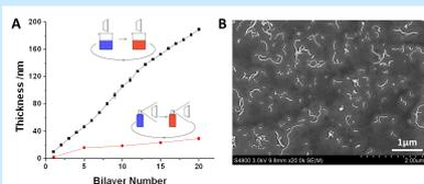
**Figure 1.** (A) Thickness of dipping and spraying (PEI/CNTs@PDA) multilayer films as a function of bilayer number. (B) SEM showed sparse CNTs spreading out over the substrate after 20 cycles of spraying LbL deposition of (PEI/CNTs@PDA) film.
