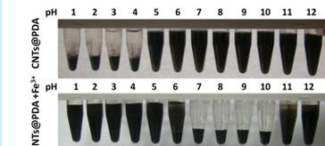
**Figure 2.** Dispersion stability of CNTs@PDA solutions in the absence (up) and presence (down) of  $\text{Fe}^{3+}$  at different pH from 1 to 12.
