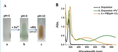
**Figure 4.** Crosslinking dopamine +  $\text{Fe}^{3+}$ : (A) the color change of dopamine solution added with 0.65 mM  $\text{FeCl}_3$  and a same volume of PEI (pH = 12, 2 mg/mL) solutions successively. (B) UV-Vis spectra of solution a, b and c.
