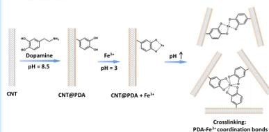
**Scheme 1.** Schematic illustration of modification of CNTs with polydopamine and the pH-dependent catechol- $\text{Fe}^{3+}$  coordination and its use in crosslinking of CNT@PDA.
