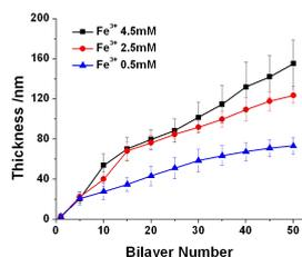
**Figure 5.** The influence of the concentration of  $\text{Fe}^{3+}$  on the growth rate of the [PEI/(CNTs@PDA+ $\text{Fe}^{3+}$ )] multilayer film. The concentration of  $\text{Fe}^{3+}$  increased from 0.5 mM to 4.5 mM.
