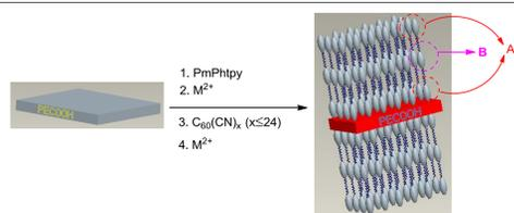
Scheme 2. Simplified Scheme of the Layer-by-Layer Self-Assembly Process for Fabrication of the Multilayer Film (PmPhtpy/M<sup>2+</sup>/C<sub>60</sub>(CN)<sub>x</sub>/M<sup>2+</sup>)<sub>10</sub>×<sub>4</sub>
