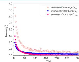
Figure 4. Temperature dependence of magnetization (M) for the films (PmPhtpy/Ni<sup>2+</sup>/C<sub>60</sub>(CN)<sub>x</sub>/Ni<sup>2+</sup>)<sub>10</sub>×<sub>4</sub>, (PmPhtpy/Co<sup>2+</sup>/C<sub>60</sub>(CN)<sub>x</sub>/Co<sup>2+</sup>)<sub>10</sub>×<sub>4</sub> and (PmPhtpy/Co<sup>2+</sup>/C<sub>60</sub>(CN)<sub>x</sub>/Ni<sup>2+</sup>)<sub>10</sub>×<sub>4</sub> at H = 30 kOe.
