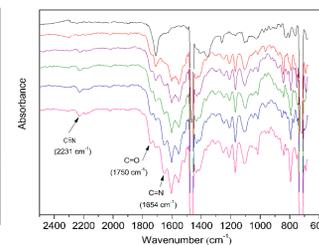
Figure 2. ATR-IR spectra of PE-COOH and the multilayer film (PmPhtpy/Ni<sup>2+</sup>/C<sub>60</sub>(CN)<sub>x</sub>/Ni<sup>2+</sup>)<sub>n</sub>×<sub>4</sub> (n = 2, 4, 6, 8, 10).
