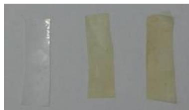
Figure 1. Photograph (from left to right) of the HDPE film and the magnetic multilayer film (PmPhtpy/Ni<sup>2+</sup>/C<sub>60</sub>(CN)<sub>x</sub>/Ni<sup>2+</sup>)<sub>n</sub>×<sub>4</sub> (n = 6, 10).
