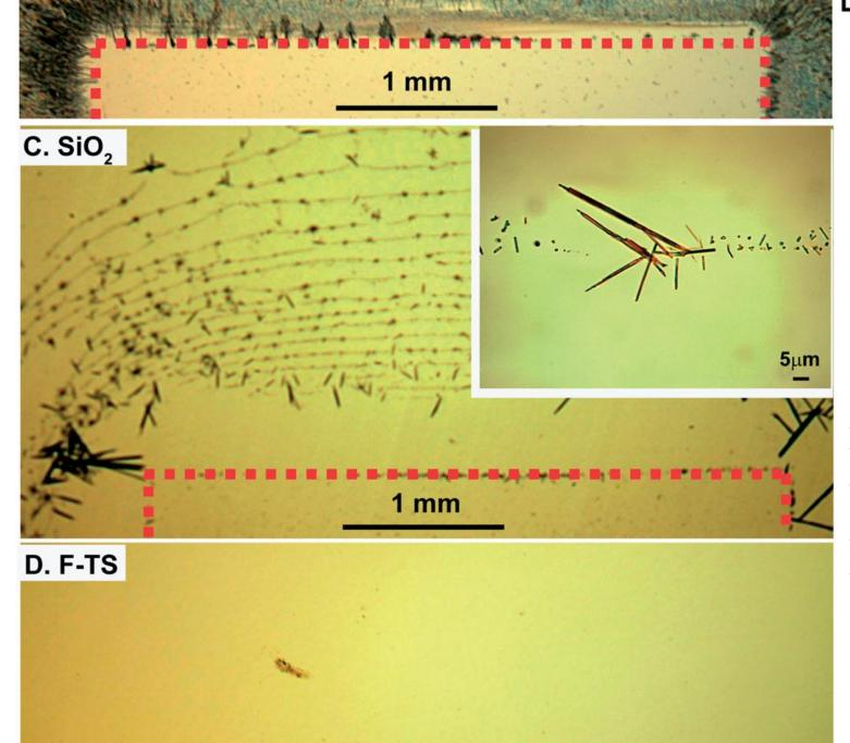
Substrates left are modified with CN-TS silane (B), bare SiO<sub>2</sub> (C), and modified with F-TS silane (D). CN-TS modified substrate has better wettability than the other two, thus better crystal attachment and alignment were obtained from 0.4 mg/mL C<sub>60</sub> m-xylene solution.
