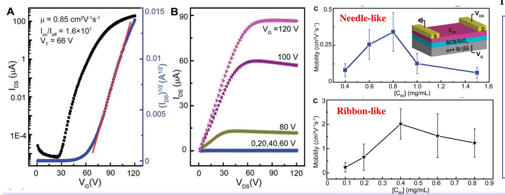
the steps formed on the bottom of the crystals. While in the ribbon-like case, with the increasing concentration, the increase in ribbon width and height result in decreasing and increasing contact resistance respectively. The interplay of these opposite effects resulted in the maximum mobility at the intermediate width (8.2  $\pm$  3.4 mm) and height (57  $\pm$  7 nm) of the ribbons.
