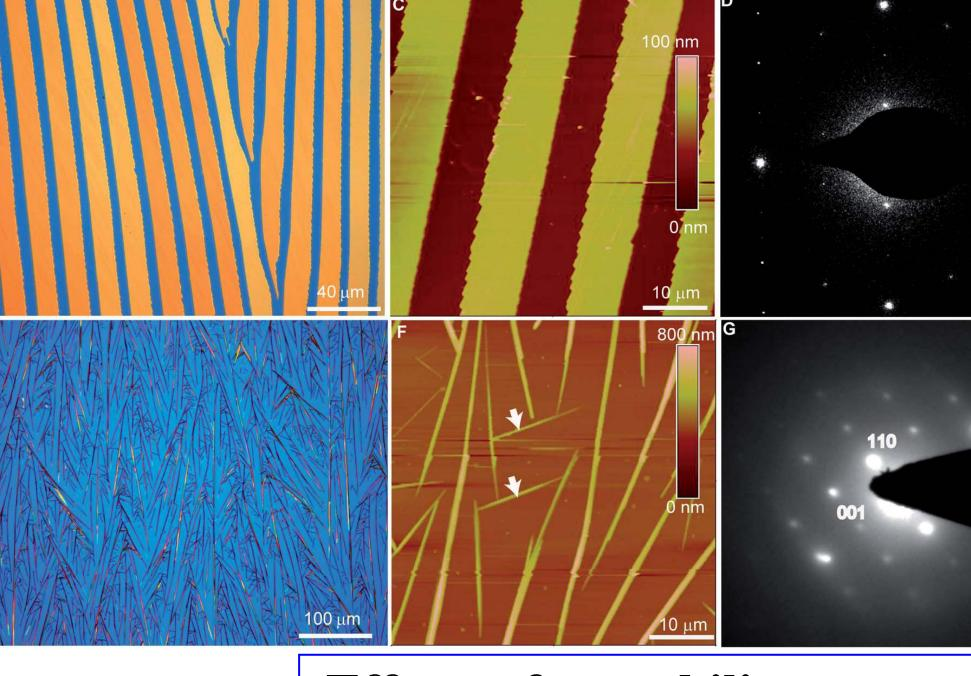
With a typical concentration of 0.4 mg/mL in different solvents, well-aligned ribbon-like (mix solvent of m-xylene and  $CCl_4$ ) and needle-like (m-xylene)  $C_{60}$  crystals were obtained in-situ on the FET substrates.
