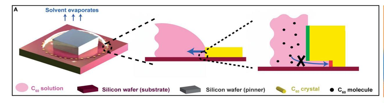
Schematic presentation of the droplet-pinned crystallization (DPC) method where a droplet of  $C_{60}$  solution is pinned by a silicon wafer. While the solvents evaporate,  $C_{60}$  crystals nucleate near the contact line of the droplet and grow along the receding direction towards the center, resulting in aligned crystals.
