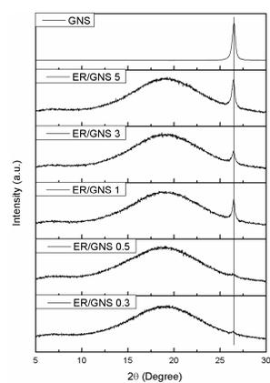
In ER/GNS, large and flat graphene flakes exfoliated, while some aggregations still exist.
