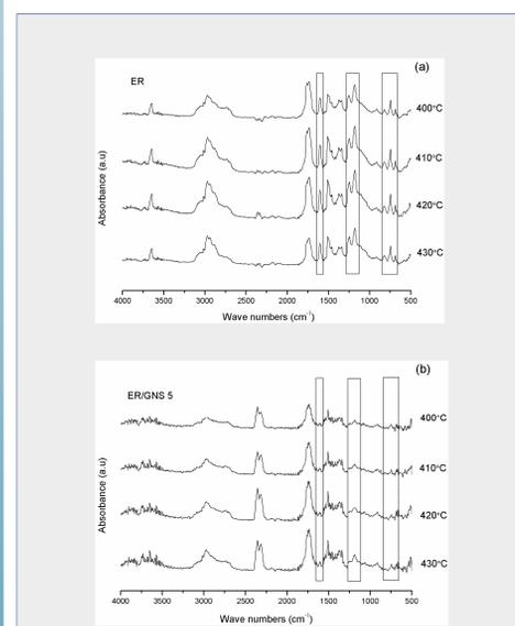
FTIR spectra of gas products at 400-430°C.
