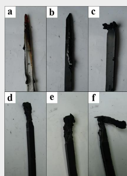
Samples after LOI tests: (a) ER, (b-f) ER/GNS 0.3, 0.5, 1, 3, 5.
